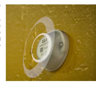
This solution makes it possible to locate the forklift truck in the warehouse and record its movements. The tag makes it possible to know the departure and arrival points of the logistic equipment and thus to calculate its travel time. This creates a great possibility to optimize and automate inventories.
